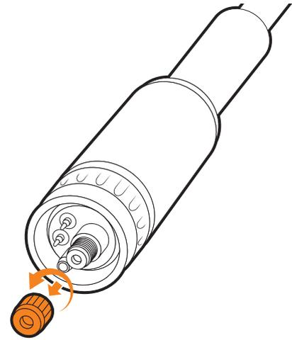
3 Carefully pull out and completely remove the existing liner. Ensure MIG torch is completely unravelled until setup is complete.
