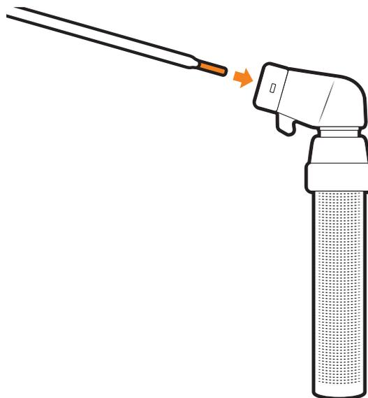
7 Twist electrode holder to tighten and securely grip electrode.
