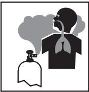
**Gas build-up.** The build-up of gas can cause a toxic environment, deplete the oxygen content in the air resulting in death or injury. Many gases used in welding/cutting are invisible and odourless.
