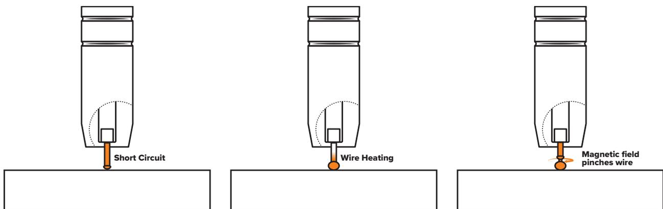
The wire approaches the workpiece and touches the work, creating a short circuit between the wire and the base metal, because there is no space between the wire and the base metal there is no arc and current flows through the wire.
