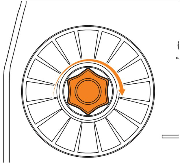
**11** Feed wire through the inlet guide tube through to the outlet guide tube. Ensure that the wire passes through the roller.
