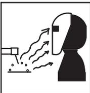
**Arc rays: harmful to people's eyes and skin.** Arc rays from the welding/cutting process produce intense visible and invisible ultraviolet and infrared rays that can burn eyes and skin.
