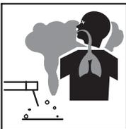
**Fumes and gases are dangerous.** Smoke and gas generated while welding or cutting can be harmful to people's health. Welding produces fumes and gases. Breathing these fumes and gases can be hazardous to your health.
