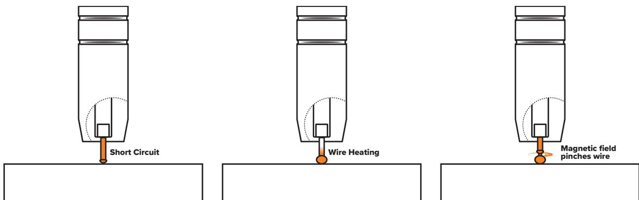
The pinch causes the forming droplet to separate and fall towards the forming weld pool.
