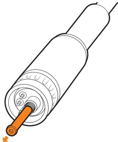
4 Carefully feed in the new liner down the torch lead all the way to exit the torch neck.
