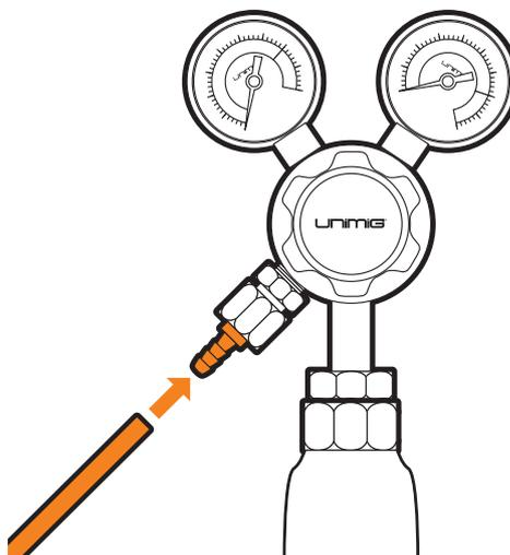
19 Adjust gas flow to 8-12L/min.
