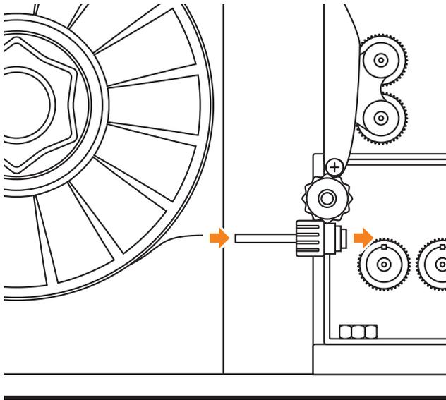
**12** Lift roller tension knob to lock wire in place. Twist to tighten.
