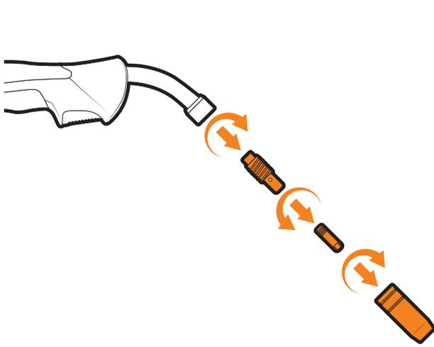
2 Remove the liner retaining nut.
